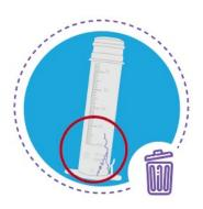
The cylinder becomes brittle or cracked or mineral deposits inhibit plunger movement
